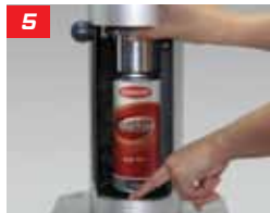
5 Secure the aerosol can into the filling machine and close the door
