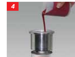
4 Fill the mixed paint into the cylinder
